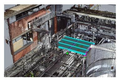
Point cloud of the space in BPL's plant where Courts Engineering custombuilt a platform to take a 37-ton machine. The machine and the platform were lowered through the roof to fit precisely among the pipe network.
