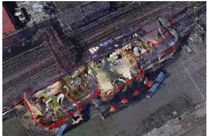
Arena4D’s animation features have enabled Sophie to strip away the exterior of the building in the animation, revealing the structure within.
