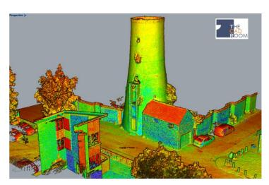
Colourised point cloud of a windmill and the adjoining building, used as part of a restoration project of the grade 2 listed building.
