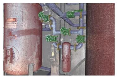
Using Point Clouds for Rhino, Veris created a highly detailed 3D model of this machinery with key elements such as joints and valves colourised. Here you can see the 3D image layered over the original point cloud.
